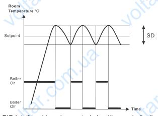
PID intelligent learning control algorithm periodically switches on and off the heating system. The period time (T) and pulse length (P) of the control signal (PWM) are determined by the setpoint and the measured room temperature.
